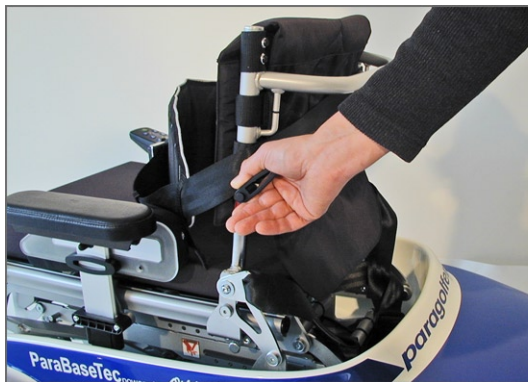
Fig. 9 Loosening the clamps and adjusting the back rest height
