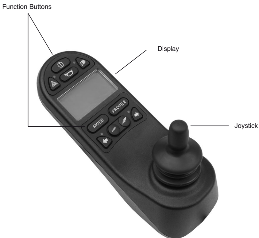
Control Panel Overview
