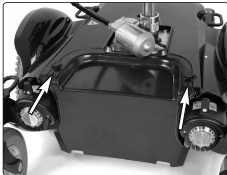
The front cover is fitted with two knobs.
