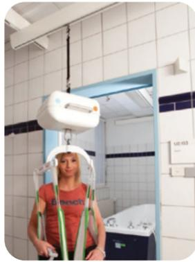
The lifting module has to be positioned close to the door header...
