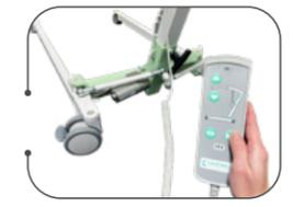
Electrical leg spreading via remote control
