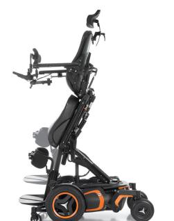
Articulating power footplate programmable footplate to fine tune height for ideal standing position
